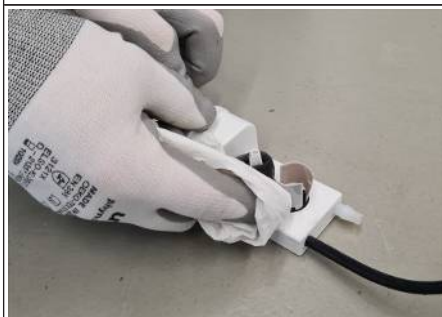
Fig. 45: Cleaning the condensate pump
