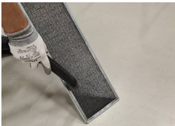
Fig. 43: Vacuum the filter and re-fit it after cleaning.
