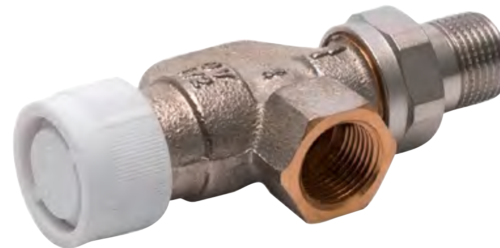
Thermostatic valve body: DN15, 1/2", axial form, NPT M30x1,5, Type 1275402
