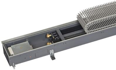
The **Katherm** QK comes in a series of different electrical versions. Connect it via a terminal strip in the electrical junction box. This is located on the side of the **Katherm** QK's water connection. Wire the unit as per the wiring diagram, which is different for each version.
