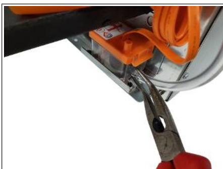
Fig. 42: Loosening the wire clip
